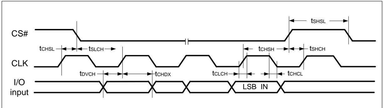
Figure 18 Serial Input Timing
