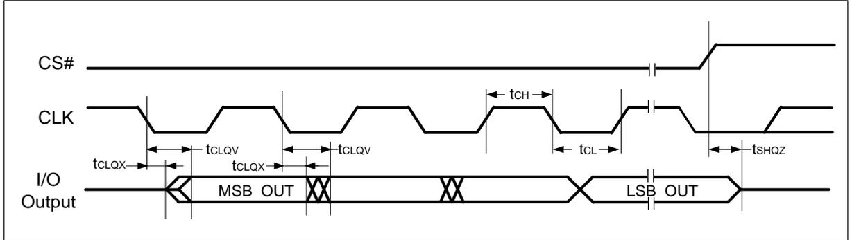
Figure 17 Serial Output Timing
